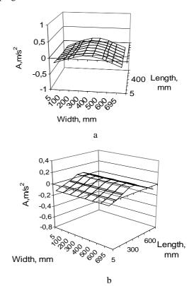
Fig. 2. Vibration modes of the square oak glued-up panel: a - across the grain, b - along the grain
