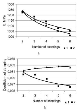
**Fig. 4.** Consistent patterns of varying average modulus of elasticity (a) and damping coefficient (b) of oak wood scantlings, and of the first-type panels made of them  $(T_{acr21}, T_{acr22}, T_{acr23})$ : 1 - for scantlings, 2 - for panels
