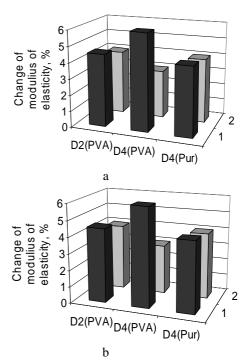
**Fig. 5.** Consistent patterns of varying average modulus of elasticity (a) and damping coefficient (b) when using adhesives of different brands: 1 – along fiber; 2 – across fiber
