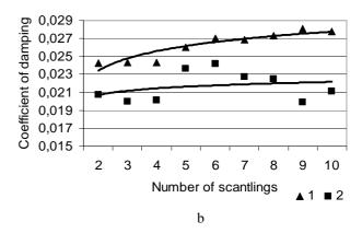
**Fig. 3.** Consistent patterns of varying average modulus of elasticity (a) and damping coefficient (b) of oak wood scantlings, and of first-type panels made of them  $(T_{all1},\ T_{all2},\ T_{all3})$ : 1- for scantlings, 2- for panels
