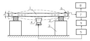
**Fig. 1.** Set-up for testing wood articles: 1 – wood assortment and its mode; 2 – elastic elements; 3 – massive supports; 4 – acoustic vibrator; 5 – generator of electric oscillations; 6 – sensor; 7 – measuring device; 8 – oscillograph; 9 – phasometer
