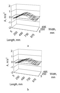
**Fig. 6.** First vibration modes of glued-up panels along grain: a – panel of 5 scantlings (f = 152.2 Hz); b – panel of 11 scantlings (f = 159.6 Hz)
