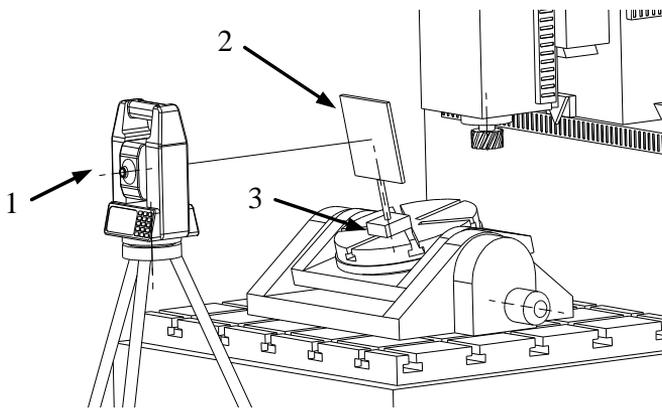
**Fig. 4.** Example of testing/calibration of rotary table of industrial milling machine: 1 – scanning instrument, 2 – milling machine, 3 – turn table (4<sup>th</sup> and 5<sup>th</sup> coordinate)
