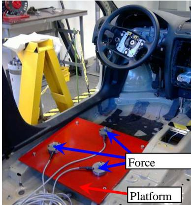
Fig. 7. Load cells (GTM)
