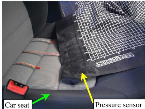
Fig. 8. Pressure sensor (XSensor)
