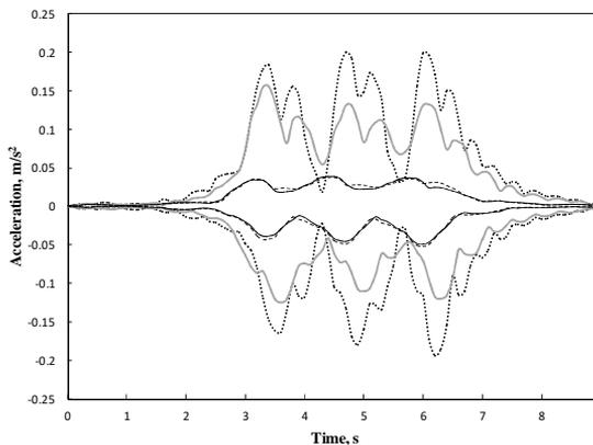
**Fig. 8.** Schematic acceleration response in a node located at 2 m from an in-filled concrete trench:
