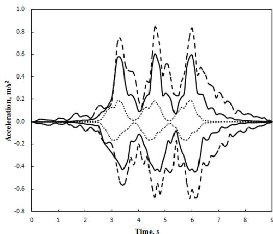
**Fig. 6.** Schematic acceleration response in a point located 1,20 m from the rail for different  $\beta$  Rayleigh coefficient: - - -,  $\beta_1 = 0.0001$ ; —,  $\beta_3 = 0.001$ ; ..... ,  $\beta_4 = 0.01$
