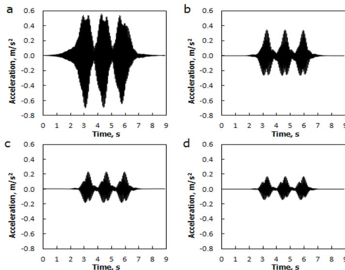
**Fig. 5.** Acceleration response in a point located at 1.20 m distance from the rail for different sand Young's modulus values ( $E$ ): a)  $E_1 = 1.7 \cdot 10^7$  Pa; b)  $E_2 = 7 \cdot 10^7$  Pa; c)  $E_3 = 12.3 \cdot 10^7$  Pa; d)  $E_4 = 17.5 \cdot 10^7$  Pa
