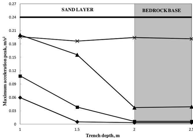
**Fig. 12.** Maximum acceleration peaks on a node located at 2 m from the trench: ———, no trench located; X, polyurethane in-filled trench; ▲, concrete in-filled trench; ■, open trench; ◆, sheet piling trench
