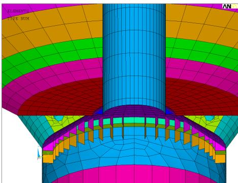
Fig. 1. Detail of mesh – tank bottom
