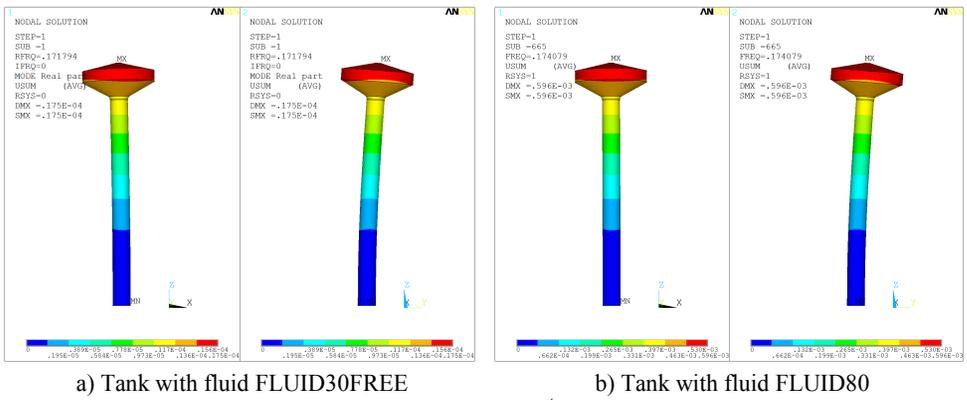
Fig. 7. Eigen mode corresponding to 1<sup>st</sup> mode of fluid movement
