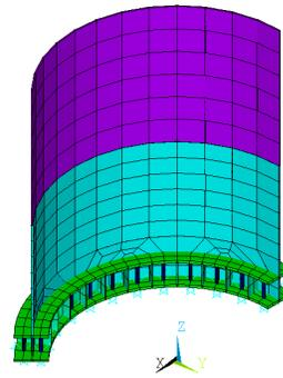
**Fig. 4.** Detail of mesh – bottom rims
