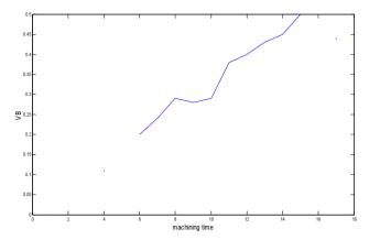
Figure 3. Tool wear VB over time.
