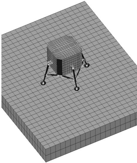
**Fig. 4.** Finite element model for soft-landing impacting
