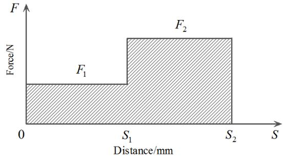
**Fig. 5.** Undergone sketch of the two-stage honeycomb buffering
