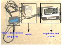
Fig. 2. TC-4850 blasting vibration monitoring system
