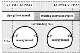
Fig. 3. Arrangement of subway tunnel vibration monitoring points
