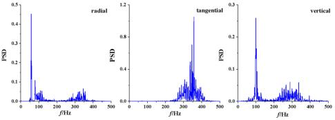
Fig. 5. The power spectral density of vibtration signals in different orientations of point 1
