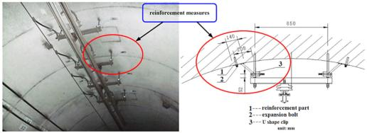
Fig. 8. The reinforcement measures of metro catenary
