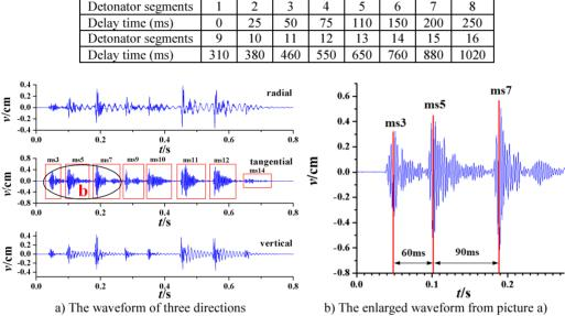
**Table 4.** The delay time of every detonator segment [10]
