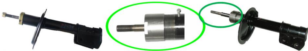
Fig. 3. Typical front shock absorber (left) and after modification (right)
