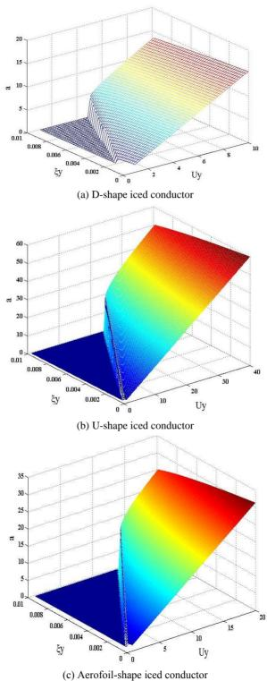
(c) Aerofoll-shape iced conductor **Fig. 8.** Galloping equivalent amplitude vs. damping ratio and reduced wind velocity for the three ice-shape conductors
