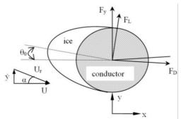
Fig. 1. Galloping analysis model of an iced conductor
