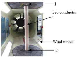
Fig. 3. A typical photo in the tunnel test
