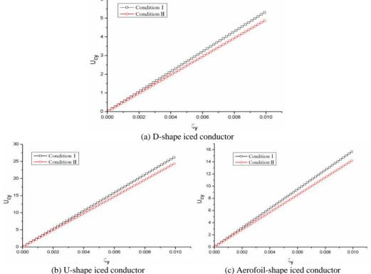
Fig. 6. Galloping critical wind velocity vs. damping ratio for the three ice-shape conductors
