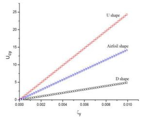
Fig. 7. Contrast on galloping critical wind velocity with the three ice-shape conductors
