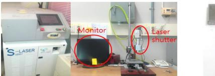
Fig. 10. Laser welding machine set-up
