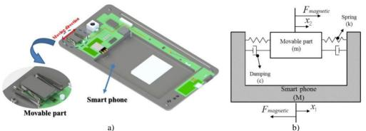
Fig. 3. a) Schematic diagram of smart phone equipped with a horizontal linear vibrating actuator, b) free body diagram of the horizontal linear vibrating actuator
