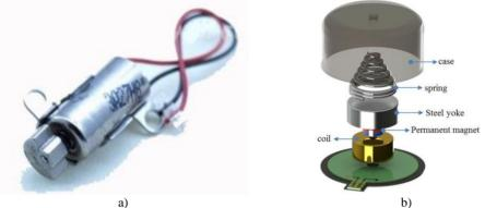
Fig. 1. Vibration actuator for a smart phone: a) bar type, and b) vertical linear vibrating actuator
