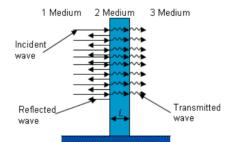
Fig. 1. Scheme of sound transmission from the first medium to the third through the second medium
