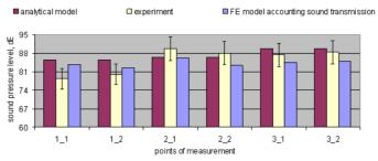
Fig. 5. Values of sound pressure in different points in the testing laboratory when the excitation of 1000 and 2000 Hz is used at the same time. The measured experimental results are given with ±5% (I) error bars (the arrangement of measurement points is shown in Fig. 4)
