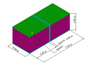
Fig. 2. FE model of closed spaces separated by the wall
