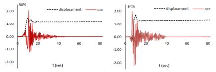
Fig. 10. Acceleration (ground motion) and displacement corresponding to achieved response spectra
