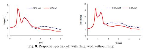
The Fast Fourier Transform (FFT) of the accelerations (concerning the response spectra shown in Figure 8) is carried out and demonstrated in Figure 9. The difference between the FFT Amplitudes in low frequency range (long period) can justify the difference between the response spectra at Figure 8.
