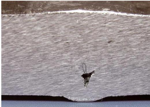
Fig. 6. Photo of the cross-section of weld joint with inner cavity discovered in it
