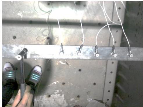
Fig. 8. Set up of measurement sensors and impact hammer
