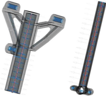
Fig. 6. FEM models of flexible main fitting and shock tube
