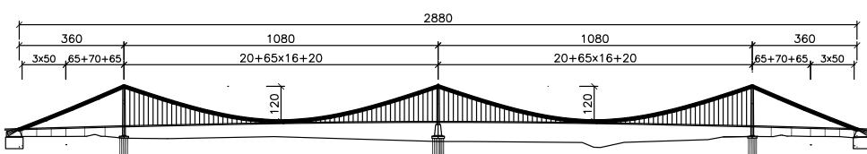
Fig. 1. General layout of Ma'anshan Yangtze River bridge (unit: m)
