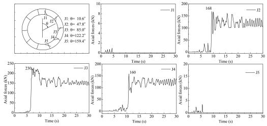
Fig. 15. Axial force in bolts at joints
