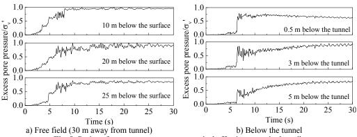
Fig. 8. Ratios of excess pore pressure to vertical effective stress in the soils
