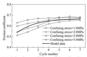
Fig. 5. Variation of average friction coefficient with cycle number
