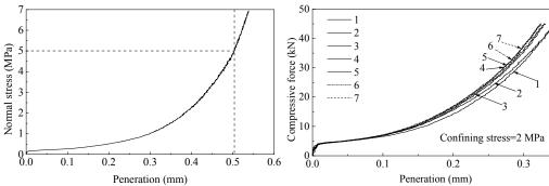
Fig. 1. Normal stress-penetration curves
