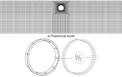
b) Concrete interfaces and bolts at joints **Fig. 6.** Numerical model
