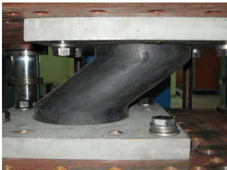
Fig. 3. Specimen under shear loading
