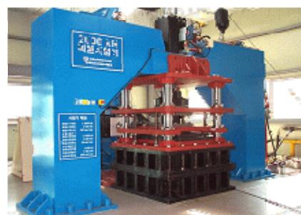
**Fig. 2.** Compression-shear test machine
