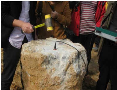
a) Low-strain integrity test
