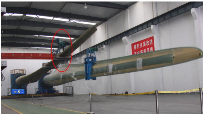
Fig. 7. Wind turbine blade fatigue loading test
