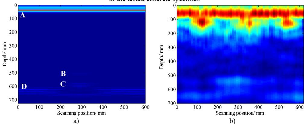
**Fig. 5.** a) The SAFT imaging result using simulation data; b) The SAFT imaging result using experimental data
