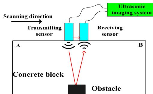
**Fig. 1.** The operation principle of ultrasonic imaging system
