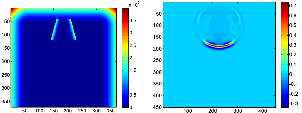
**Fig. 2.** The distribution of attenuation factors with the mobile PML absorbing boundary
