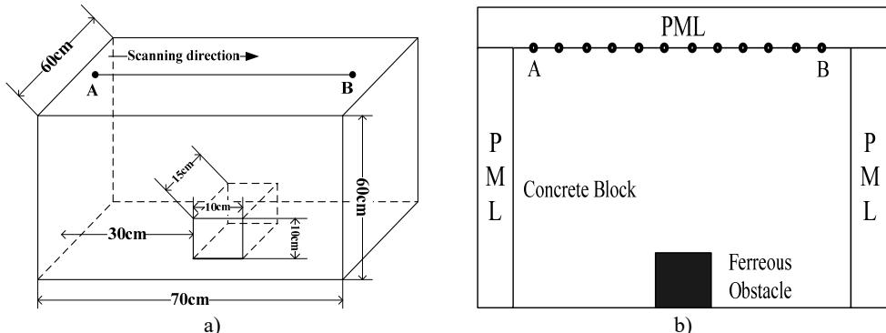
**Fig. 4.** a) The configuration of the tested concrete specimen; b) the cross-section of the tested concrete specimen
