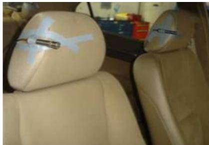
Fig. 1. Microphone positions for testing the interior noise
