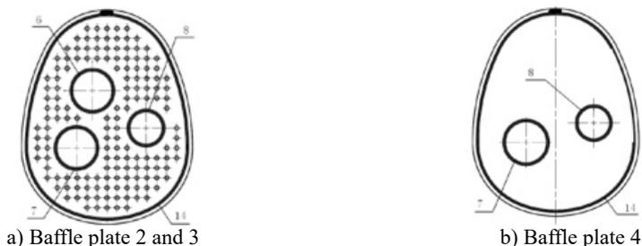
Fig. 14. Sectional view of the baffle plate
