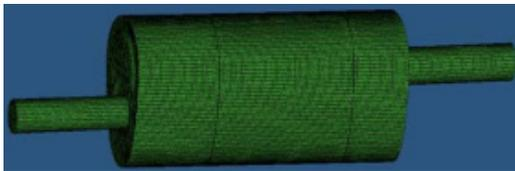
Fig. 6. FEM of muffler meshes
