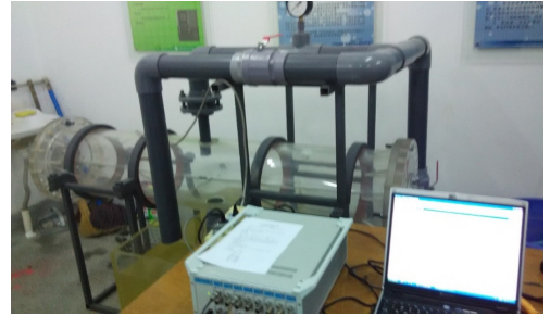
a) The schematic diagram b) The experimental device Fig. 20. The vibration test device for flexible pipe in a cylindrical fluid domain
