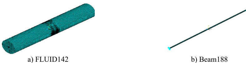
Fig. 3. The fluid-structure coupling FEM model of flexible pipe in cylinder fluid domain
