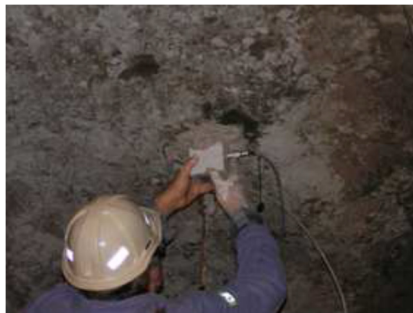
Fig. 1. Location of accelerometer in copper-ore mine
