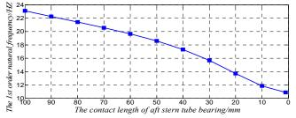
Fig. 10. The influence of effective contact length of aft stern tube bearing on the 1st order natural frequency
