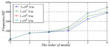
Fig. 8. The influence of intermediate bearing stiffness on the natural frequencies of shaft
