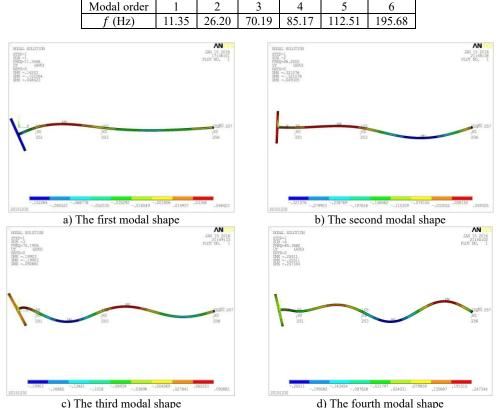
**Table 2.** The natural frequencies of propulsion shafting test rig
