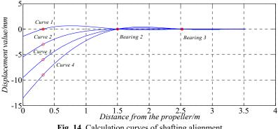
Fig. 14. Calculation curves of shafting alignment
