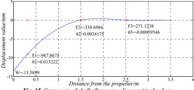
Fig. 15. Curve axis of shaft after curve alignment technology
