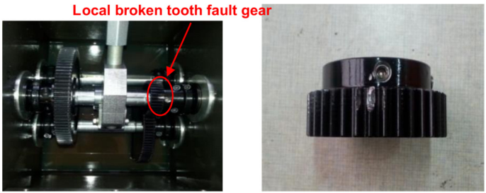
Fig. 3. Local broken tooth fault gear
