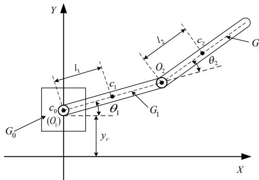
**Fig. 1.** Simplified model of the 2-DOF manipulator
