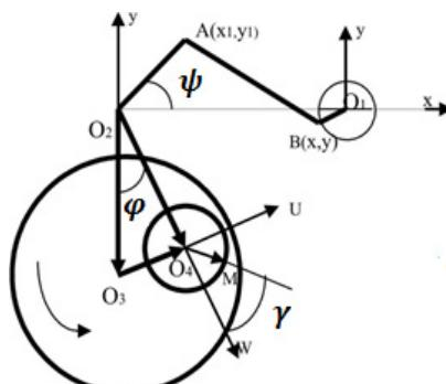
Fig. 1. Schematic diagram of the grinding mechanism
