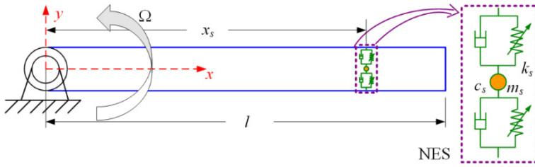
**Fig. 1.** Rotating nonlinear beam coupled with a NES
