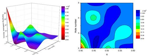
Fig. 12. Damping coefficient of square orifices with respect to the tightness factor and orifice number
