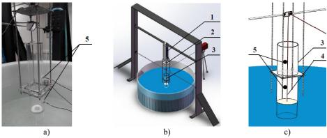
**Fig. 4.** a) A photograph of the experimental device; b) a schematic of the experimental device; c) a dual-chamber air spring
