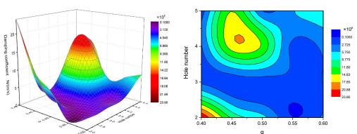
Fig. 9. Damping coefficient of circular orifices with respect to the tightness factor and orifice number
