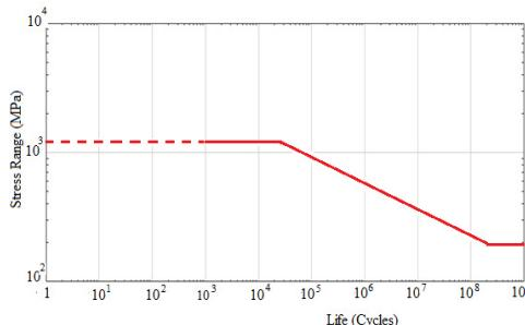
**Fig. 3.** 35CrMoA Steel material S-N curve (NASTRAN program window)
