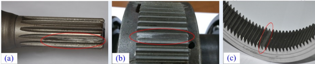
Fig. 6. Implanted wear fault: a) sun gear, b) planet gear, and c) ring gear
