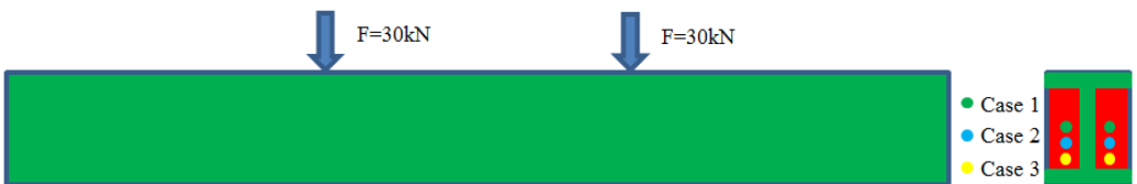
Fig. 5. Pre-stressed concrete beams under different eccentricities
