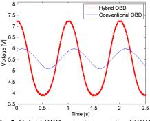
Fig. 5. Hybrid OBD against conventional OBD with the same conditions of optical power
