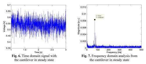
In the presence of a frictional force, the natural frequency oscillation is determined by the ratio between the damping factor  $\delta$  and the cantilever natural frequency  $\omega_n$  in radians per second. Oscillations with periodic and exponentially decreasing amplitude means  $\omega_n > \delta$ . Then, a frictional force is introduced in the fixed end of the cantilever, as shows Fig. 8, and there is an
