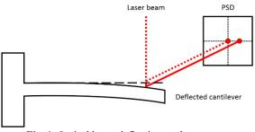
Fig. 1. Optical beam deflection readout system
