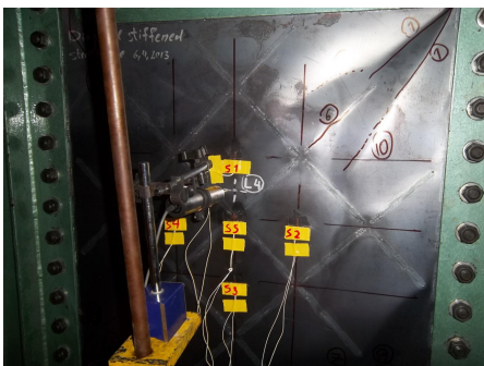
Fig. 12. Nodal buckling lines for DS-SPSW
