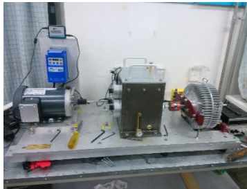
Fig. 3. Bearing fault simulation test bench
