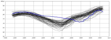
Fig. 11. Results comparison from EOL - amplitude of second harmonic frequency
