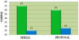
Fig. 13. Amplitudes of sound pressure comparison: green – first harmonic frequency, blue – second harmonis frequency
