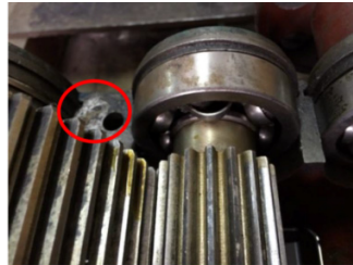
b) Bearing cage fracture
