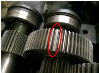
a) Gear broken tooth
