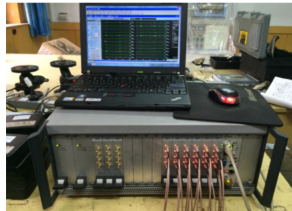
Fig. 4. The gearbox fault diagnosis test system
