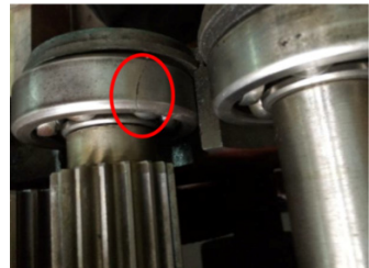
c) Bearing outer ring crack
