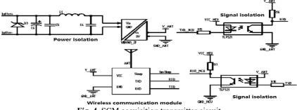
Fig. 4. SCM acquisition transmitter circuit
