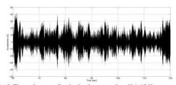
Fig. 8. The random test vibration levels measured on Ch6 (63 Hz resonance)
