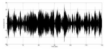
Fig. 7. The random test vibration levels measured on Ch4 (27 Hz resonance)
