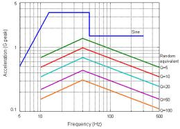
Fig. 3. Comparison of the Sine equivalents of the Random profile, with various Q. Note that for higher Q, the Sine equivalent of the Random profile has a lower amplitude
