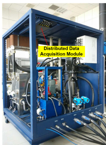
Fig. 6. The installation location of distributed data acquisition module
