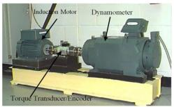
Fig. 1. Experimental setup for bearing vibration analysis
