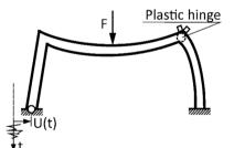
Fig. 1. A moment resisting frame under seismic excitations with two rotational sensors placed at its corner (two little squares) to monitor plastic hinge development
