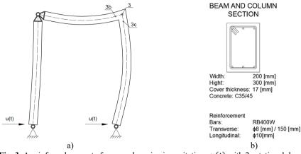
Fig. 3. A reinforced concrete frame under seismic excitations u(t) with 2 rotational degrees of freedom (3b and 3c) to monitor plastic hinge development of node 3
