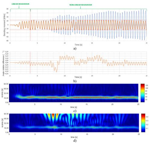
Fig. 6. Comparison of linear and nonlinear frame behavior under seismic excitations: a) linear and nonlinear bending moment in node 3, b) rotation difference between auxiliary nodes '3b' and '3c', c) wavelet map of nonlinear bending moment response with parameter 'a' standing for scale of the wavelet, d) wavelet map of the rotation difference of node 3 shown in plot (b)
