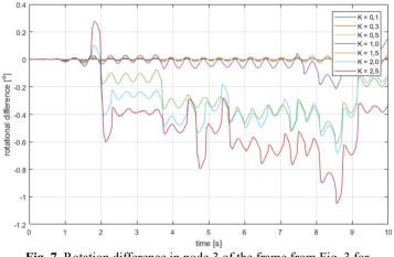
**Fig. 7.** Rotation difference in node 3 of the frame from Fig. 3 for various seismic intensities (values of the *K* multiplier changing from 0.1 to 2.5)
