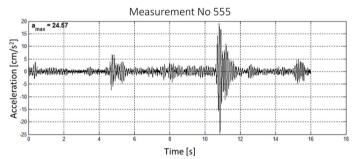
Fig. 2. Waveform recorded on the fifth floor in z direction
