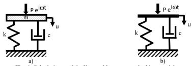
Fig. 4. Calculation model of base with mass m and without weight
