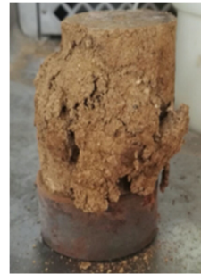
Fig. 7. Specimen after test
