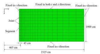
Fig. 3. The computational model for back analysis of the jointed TBM tunnel lining rigidity
