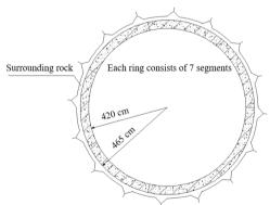
Fig. 2. Schematic diagram of the jointed TBM tunnel lining
