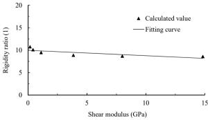
Fig. 6. The relationship between rigidity ratio and shear modulus (0.3 g)
