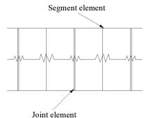
**Fig. 4.** Calculation model of rigidity ratio between segment and joint element
