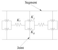
Fig. 7. Calculation model of equivalent rigidity considering rock resistance
