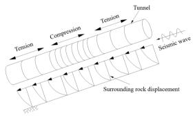
Fig. 1. A tunnel subjected to alternating tension and compression during an earthquake
