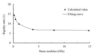
Fig. 5. The relationship between rigidity ratio and shear modulus (0.1 g)
