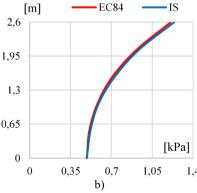
**Fig. 2.** a) The comparison of peak values of hydrodynamic impulsive pressure distribution along the canal wall height by recommendation of EC8-4 and IS, b) the comparison of peak values of hydrodynamic convective pressure distribution along the tank height by recommendation of EC8-4 and IS
