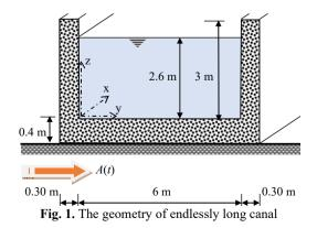
Response of open top liquid filled concrete canal was worked by using of FEMALE FSI formulation. This model was signed "Model FSI". The solid walls and base of the canal was modelled by using 2D SOLID finite element with plain strain definition and the fluid inside the canal was modelled by using 2D FLUID finite elements under plain strain definition.
