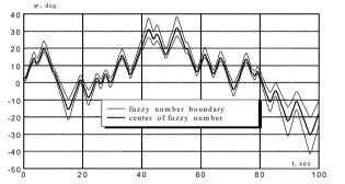
Fig. 2. Results of modeling fuzzy dynamics of underwater vehicle "AFALINA"
